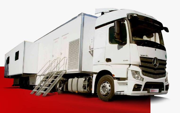
Mobile Clinic Vehicle is designed according to needs of customer. It is like a Mobile Clinic and fully equipped with medical equipments. The Hospital Trailer consist of many room as, Examination Room, Reception, Laboratory, X-Ray, Operating Room, Tecnical Room, WC and Shower Room.
